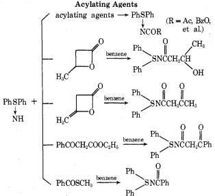
Scheme II. Reaction of Free Sulfilimine with Acylating Agents
